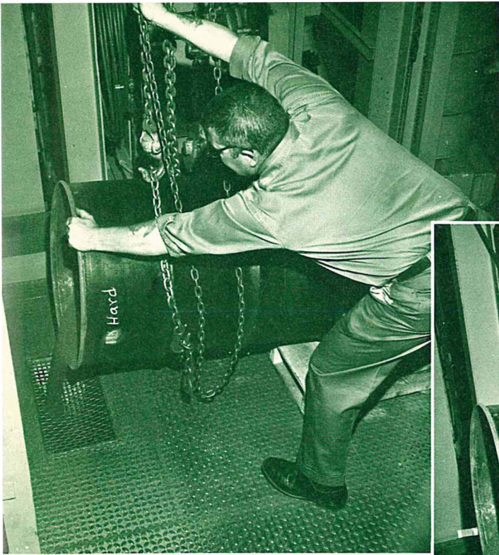
Above: Previous method had required operator to guide and balance barrel under strain while lowering by hoist. New device by operator Bill Nastos (right) now makes unloading a simple task.
